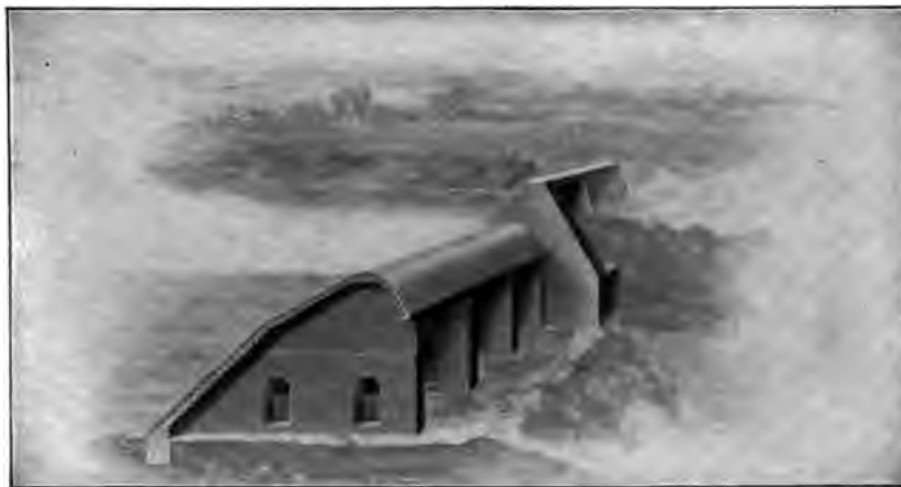
FIG. 43.—SECTION OF CONCRETE-STEEL CURTAIN-DAM.
