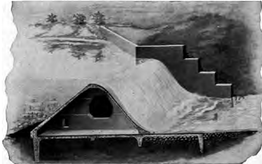
FIG. 44.—SECTION OF CONCRETE-STEEL APRON-DAM FOR CLAY OR GRAVEL FOUNDATION AND HIGH HEAD.
