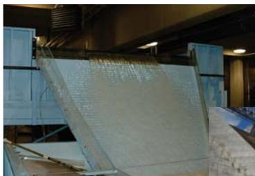
Hickory Log Creek Dam's converging 180-foot high stepped spillway was equipped with a crest gate. This approach created both construction economy and hydraulic complexity.
