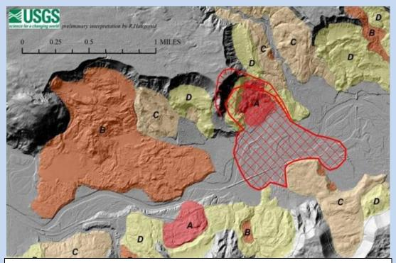
A USGS map based on interpretation of lidar data shows landslide zones in the area surrounding the March 22 slide, which is indicated by the red cross-hatched area. The zones are color-coded to indicate relative age. Red zones (also marked "A") are youngest, orange "B" zones are older, brown "C" zones are even older, and yellow "D" zones are the oldest. All of the indicated slide zones are younger than 14,000 years, when an ice sheet is thought to have retreated from the area.
