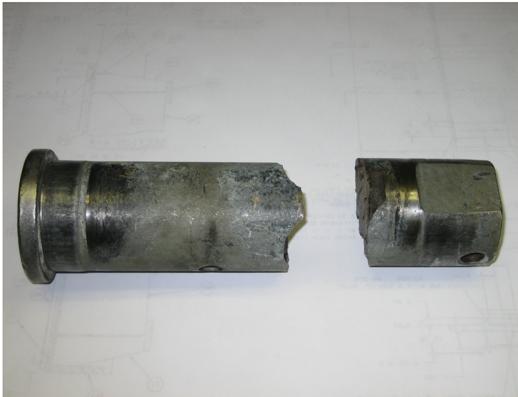
Photo 2: Wanapum Dam Tainter Gate 1, left bank hoist chain, roller pin 41
